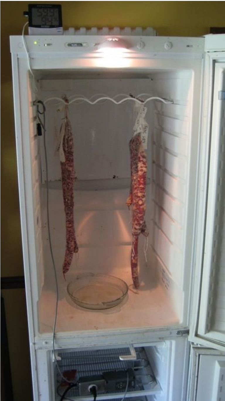
The author's salami-curing chamber, a refrigerator with an overriding temperature controller set for 57°F/14°C.
